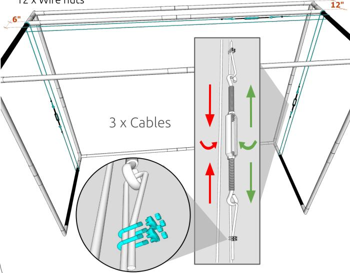
Loop 2 x SideRite cables around upper and lower depth poles 12" from back
