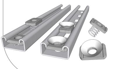
Your hardware kit may include cone or spring style strut nuts. Both work similarly. **Press** nut into channel and **twist** to hold nut in place.
