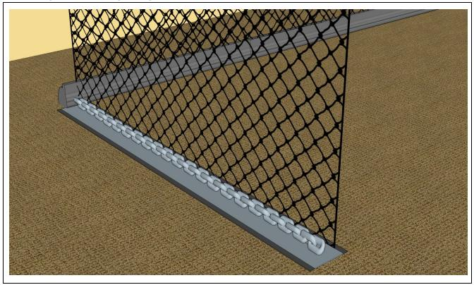
• Pull down on the netting to provide as much tension on the net as possible while bringing each edge of the pocket up on either side of the netting and attach the velcro edges of the pocket through the netting. Pocket and chain should remain in contact with the floor.
