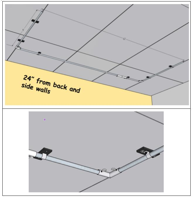
Lag screws and toggle bolts are provided to attach the brackets to ceiling. Use Lag bolts to attach to ceiling joists and toggle bolts to attach to drywall. At least one side of the ceiling bracket should be anchored to a ceiling joist.
