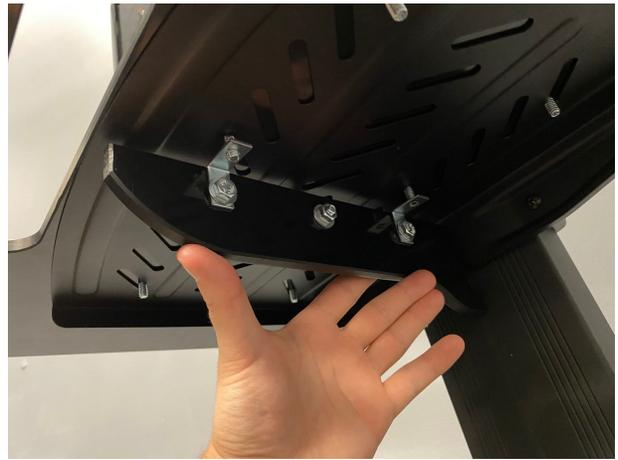
Secure the bottom supporting bracket with 3 washers and 3 nuts, one per carriage bolt
