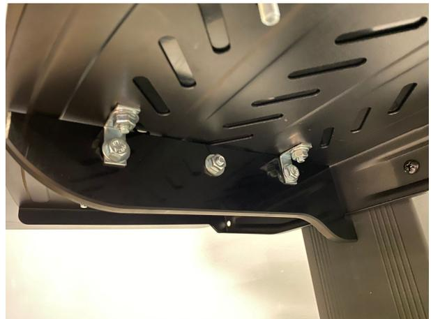
Secure the remaining 4 carriage bolts to the metal tray with 4 washers and wing nuts.
