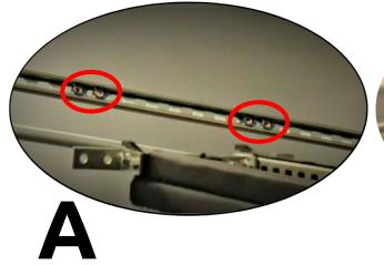
Cone nuts should be inserted (<u>Insert Cone</u> <u>Nuts</u>)
