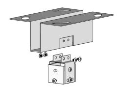
B. Attach Adapter Bracket to Projector
